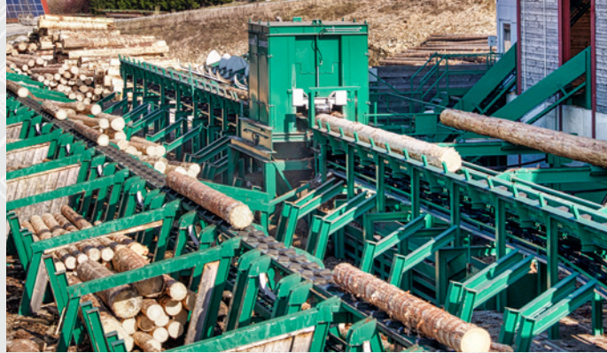
Rotor debarkers: With a passage width of 12–110 cm for logs with a minimum length of 1.60 m – with a choice of 3 or 5 debarking tools.
