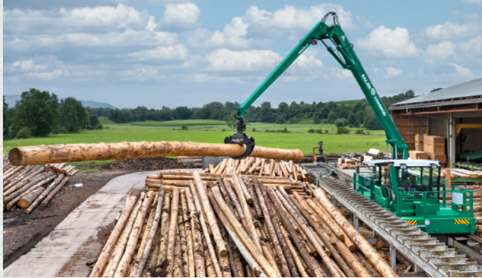
Roundwood sorting and transporting carriage (RSTW): Economical measuring, cutting, sorting, handling and feeding.
