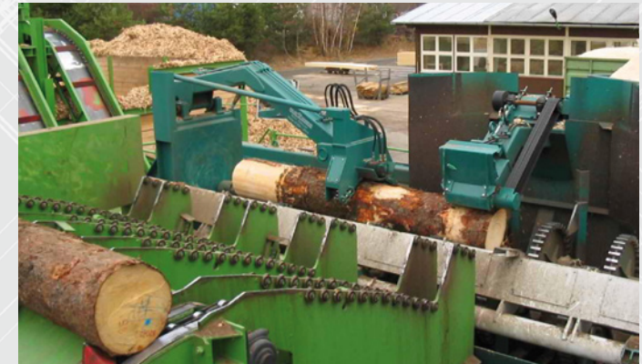
Combined machines: The combined machine saves space and costs compared to a separate cutting head debarker and reducer by bringing the functions of both units into a single machine.
