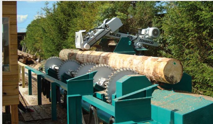
Cutting head debarkers with a wide range of applications: Inexpensive entry-level model with 180 mm rotor head up to fully automatic debarking with front-end quill clamping
