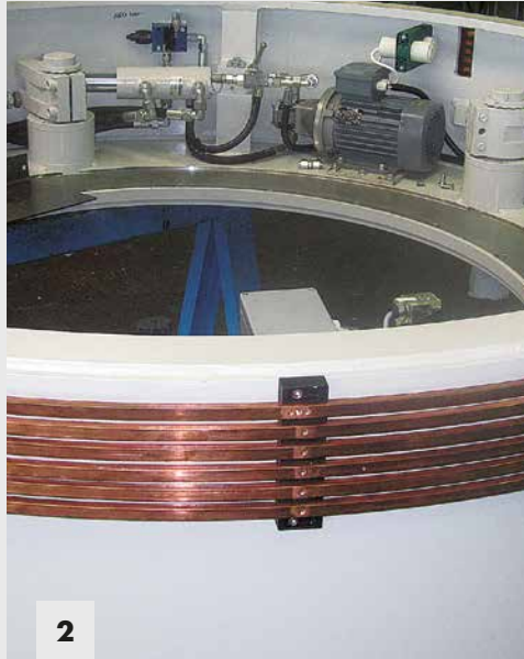
Fig. 2: Slip rings supply the unit.
