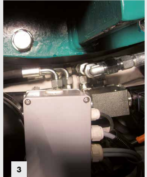
Fig. 3: A directional control valve controls the five cylinders of the blade arms, open and close. Five integrated diaphragm accumulators collect the quantity of equalisation oil for the differential cylinders. The pump draws the oil (with a rotational movement of the entire rotor) from an air-free bladder tank.
